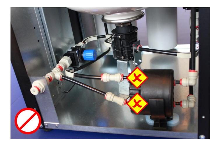
Connect the fittings with the hoses (4x) Attach the locking clips (4x) that you have saved Push the pump into its holder
